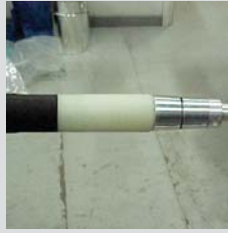
Factory prepared cable end ready for installation
