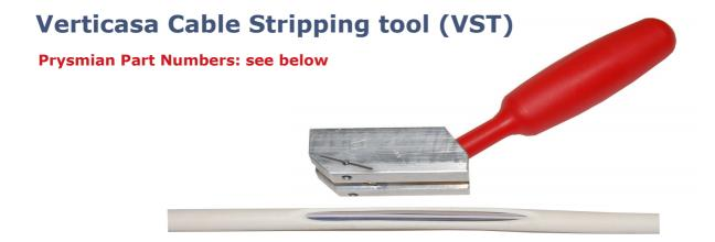
The Verticasa Cable Stripping tool (**VCST**) is typically used in multi dwelling units or office fibre cabling systems where extractable fibre cables like the Prysmian Verticasa cable range have been installed. It is used to create a longitudinal window cut on the cable. The window cut will allow to access the fibre modules inside the cable.
