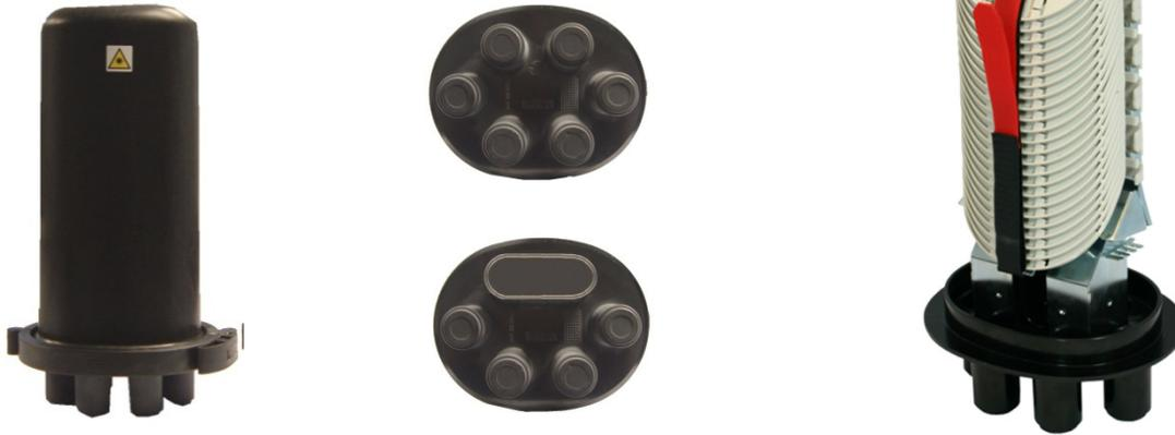
The Compact Single Circuit Joint allows the termination of up to 96 fibres (4 fibres per tray). The joint is available with either 6 circular ports or 1 oval port and 4 circular ports.
