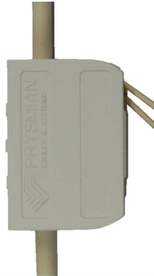
The Verticasa Mini Riser Box, is mainly used for Multi Dwelling Units (MDU's) or office fibre cabling system's. It is a compact splicing box enabling the splicing of up to 6 drop cables of 2.6mm diameter to a main in-line cable. The Mini Riser Box houses a single splicing tray.
