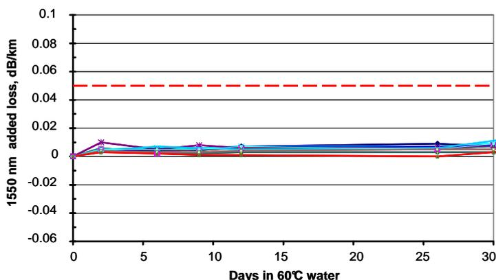
Fig. 2 Ribbon (12 fiber) watersoak test
