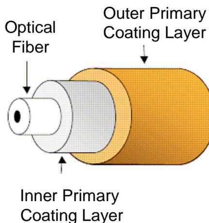
**Fig. 1** Schematic drawing of Single-Mode Fiber
