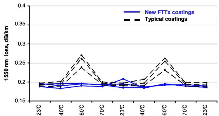
**Fig.3** Basketweave/temperature cycle results for typical commercial SM coating system (dashed) and the optimized coating system (solid).
