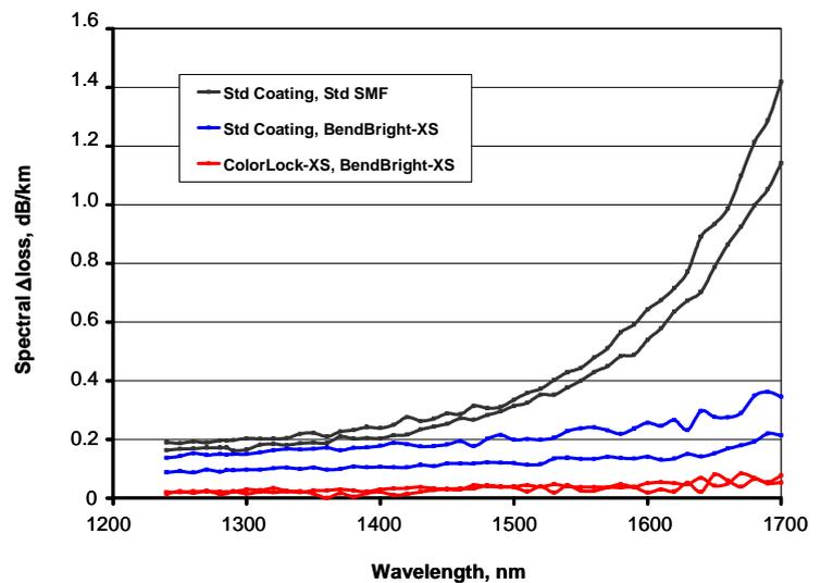
**Fig. 6** Sandpaper drum spectral micro bending test
