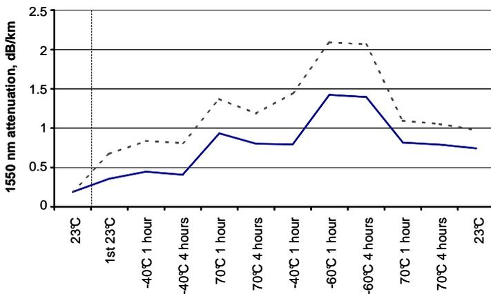
**Fig.4** Sandpaper drum/temperature cycle results for typical commercial SM coating system (dashed) and **ColorLock-XS** (solid).
