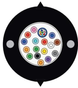
**Cable Application:** Indoor installation on cable tray, in corridors, shafts or aerial installation with 15m span. Easy selection and removal of a tube for tapping and connection at the floor. The fully dry flexible micro-modules provide easier storage & faster installation and access to the fibres with specific tools and without further cleaning. The minimum strip-ability of the modules is 30 cm.
