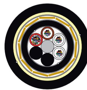
**Cable Application:** the cables are suitable for aerial installation The use a set of protection rods and helical dead end is recommended, in order to achieve the mentioned performance.
